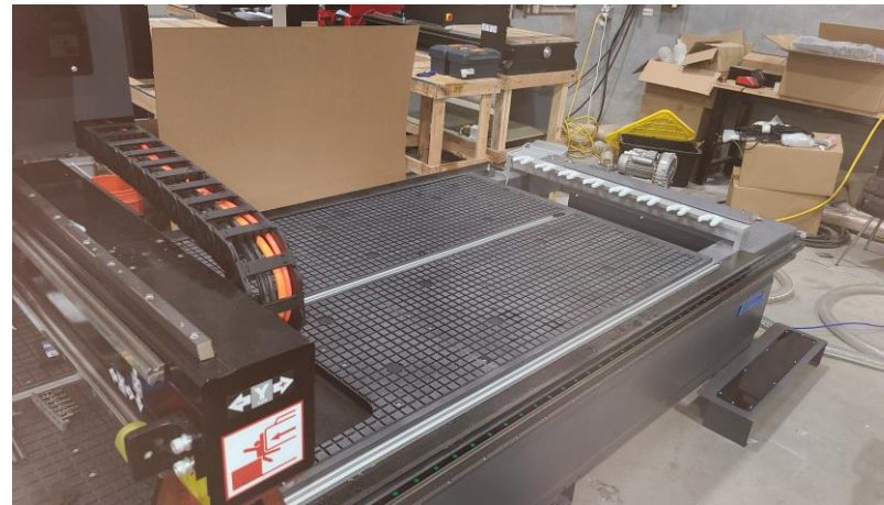
Utilize Vacuum Table along with T-Slots.
