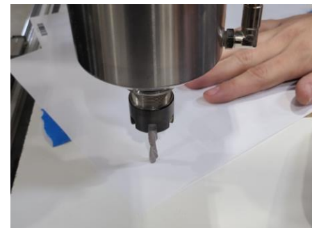
"Z-Zero Position with a piece of paper"
