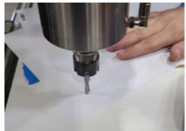
"Z-Zero Position with a piece of paper"
