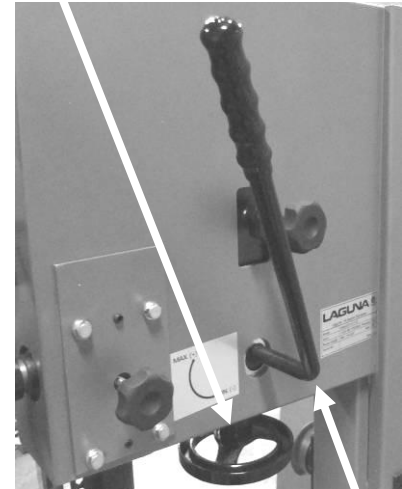
Quick action blade tension lever (activated)
