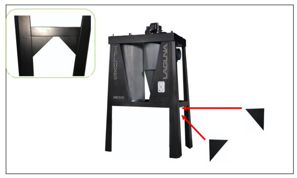
Step Seven: Secure the (2) triangular cover plates to the left side of the unit; facing the control side. Use (8) 5/16" \*1" hex bolts, (16) 5/16" \*OD18\*2t flat washers and (8) lock nuts.
