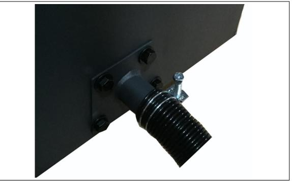
Step Twenty Five: Attach the other end of the Ø1-1/4" x0.8M black flex hose to the drum lid vacuum suction tube and use the Ø1-1/4" hose clamp to tighten and secure the black flex hose in place.
