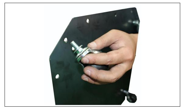
Step Nineteen: Assemble the front and back panel to the drum base using (10) 5/16" \*5/8" Philip hd bolts, (20) 5/16" \*OD18\*2t flat washers and (10) 5/16" nuts.
