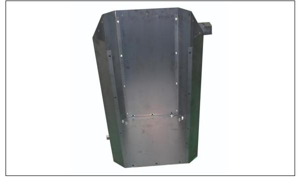
Step Twenty One: Assemble the top rim to the panels using (11) 5/16" \*5/8" Philip hd bolts, (11) 5/16" \*OD18\*2t flat washers and (11) 5/16" nuts.
