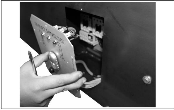
Step Twenty Eight: Insert the control panel through the hole in the side panel to place in the control box before detaching the control box.
