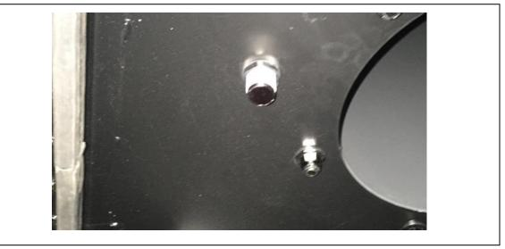
Step Fifteen: To adjust the distance of the sensor to detect the dust waste level use the white plastic pin that was provided in the hardware box.
