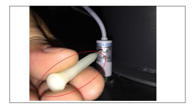
Step Twenty: Using the white plastic pin, insert the sharp point into the top end of the proximity sensor that is on top of the drum lid. You will find a small hole to on top where you can turn clockwise or counterclockwise. **%Clockwise: Lower dust waste level in drum (Less full drum) %Counterclockwise: Higher dust waste level in drum (Fuller drum)**
