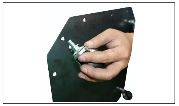
Step Twenty Two: Assemble the front and back panel to the drum base using (10) 5/16" \*5/8" Philip hd bolts, (20) 5/16" \*OD18\*2t flat washers and (10) 5/16" nuts.
