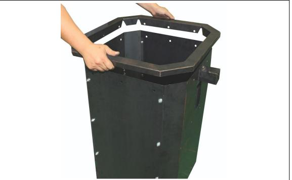
Step Twenty Five: Assemble the latch to the drum using (4) 3/16" \*3/8" round head thread bolts.
