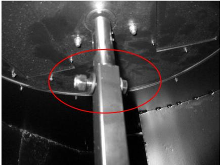
3. With the help of another person, loosen the 12 bolts holding the canister filter to the dust chute. Carefully remove the canister filter off from the dust chute.
