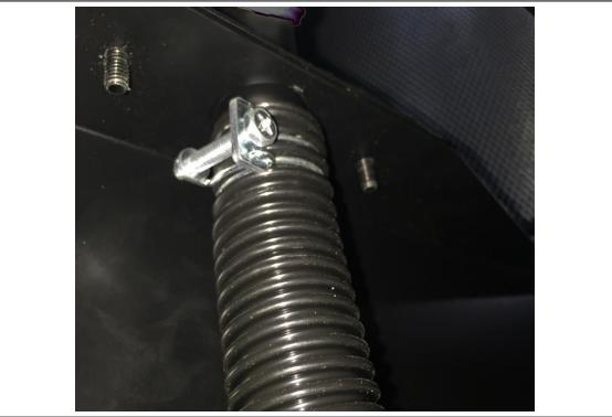
Step Twenty Nine: Place the vacuum suction ring inside before inserting the plastic bag in the Octagon drum.
