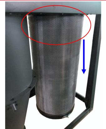
4. With the canister filter removed use a compressed air gun to thoroughly clean between the pleats, both inside and outside.
