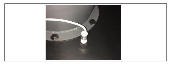
Step Eighteen: Make sure that the proximity sensor is not thread in too deeply into the drum lid. As this will create interference when the drum is inserted and may hit the proximity sensor creating damage.
