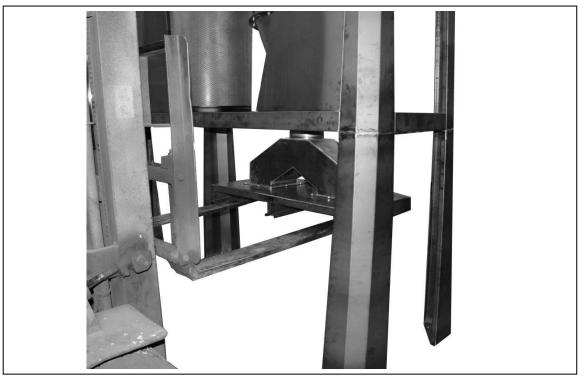
Step Fifteen: Secure the latch base plate to the front side of the drum lid using (2) 3/16" \*3/8" round head bolts.
