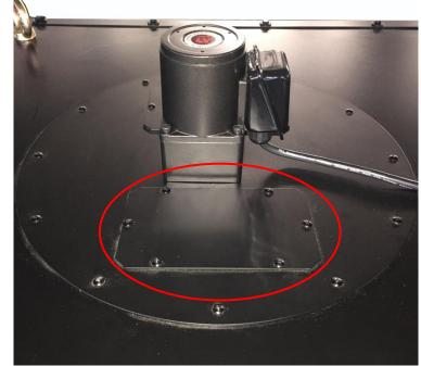
Loosen the bolt off of the rotation shaft as shown below. Set the shaft aside for later use. Keep the bolt for use when reassembling the rotation shaft.
