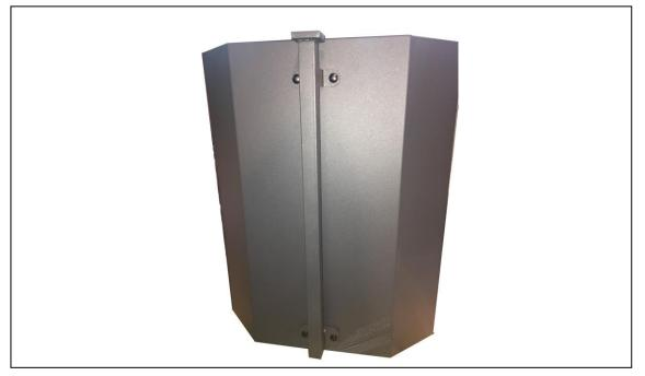
1.2. Take the one of the cover plates, (2) 1/4"\*1/2" carriage bolts, (2) 1/4"\*OD19\*2t flat washers and (2) 1/4" hex nuts and secure the cover plate to the opening on the top of the drum. For the bottom holes do the same, but first use foam tape to cover the square opening before bolting on the cover plate. Do the same to the second drum.
