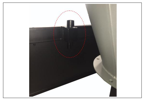
Step Nine: Take the drum lid vacuum suction tube and attach to the drum lid using (2) 1/4''\*3/4'' hex bolts and (2) 1/4''\*0D19\*2t flat washers.
