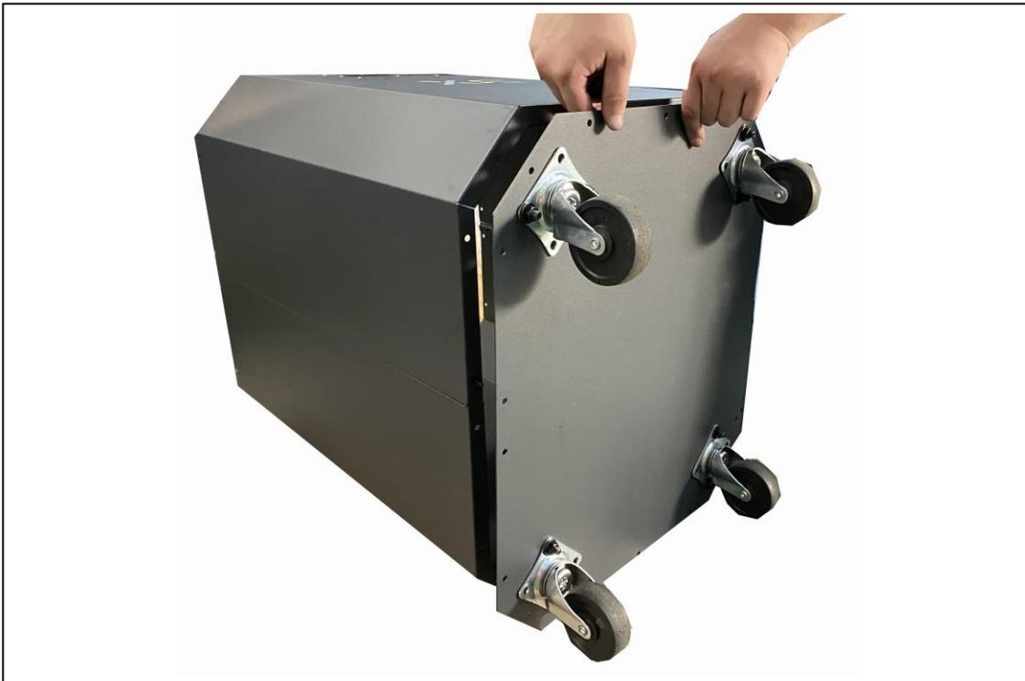
10. Place the drum upright and attach the top rim using (20) 3/16" x 1/2" Philips hd bolts, (20) 3/16" flat washers and (20) 3/16" hex nuts.
