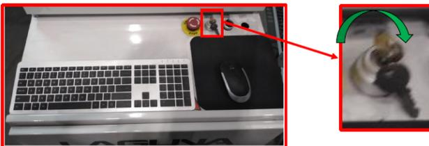
5.) Turn the Black Water Pump Switch to the right towards the “ON” Position.
