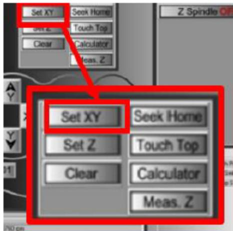
**Note:** Step 6 is not necessary to execute a 3D-Scan. If the probe needs to be repositioned at the same starting location, setting the local zero for X and Y will allow for accurate repositioning.
