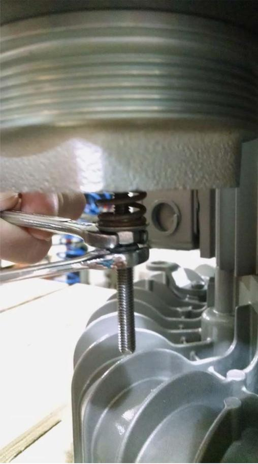
5) Reassemble the valve cover.
