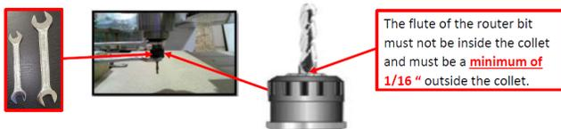
**Note:** Use this process for all other router bits that you need to fit but you will have to change the collet if the shank of the router bit is a different size.
