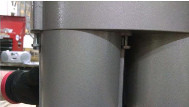
3) The valve stem will be exposed. Crack the two nuts apart and adjust the “tension nut” to achieve desired vacuum level.
