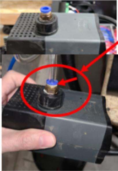
**NOTICE!** To release, the hose from the fitting, press down on the top of the blue ring on the fitting and the hose will be released.
