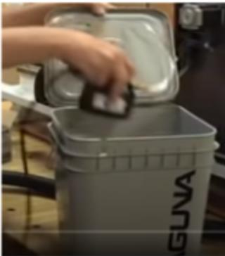
5) Place the water pump's black electrical cord (110V) into the pail's slot. Ensure that the black cord is leading to an electrical outlet.
