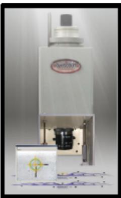
**OPTISCOUT OVERVIEW AND WORKFLOW-**The purpose of Optiscout is to compensate for deviations that arise
