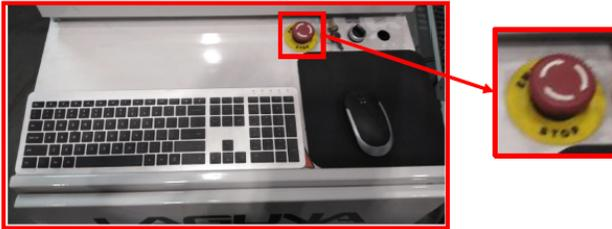
Reset after an **“Emergency Stop Button”** – Rotate the **“Emergency Stop Switch”** Clockwise a 1/4 turn.
