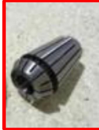
**Note:** The Collets and Spindle Collet Hole must be cleaned regularly. Ensure that the slots in the Collets are free of sawdust as sawdust builds up and will stop the Collet from compressing. If the Collet or Spindle Hole are not clean, the router bit may not run true, and this will affect the performance of your machine.
