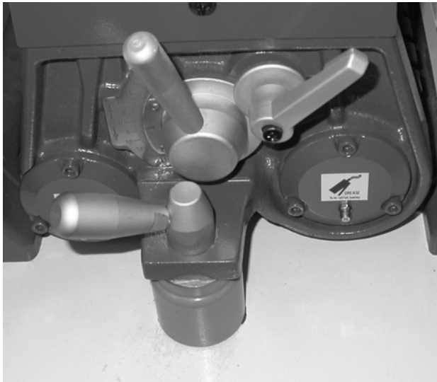
Clamp and spacer assembled
