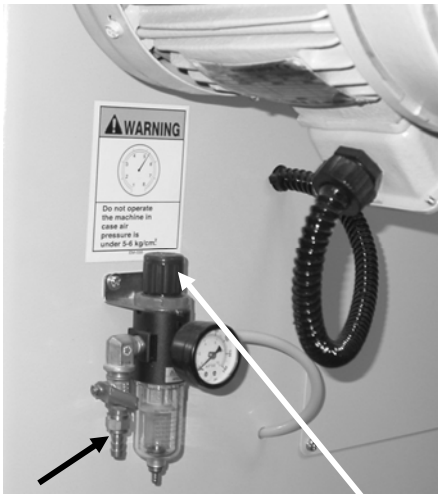
Air line connection
