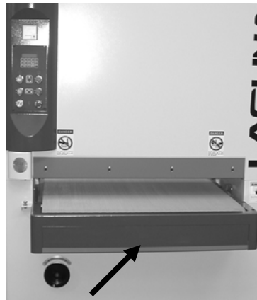
Bed safety switch
