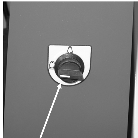
Sanding belt tension switch
