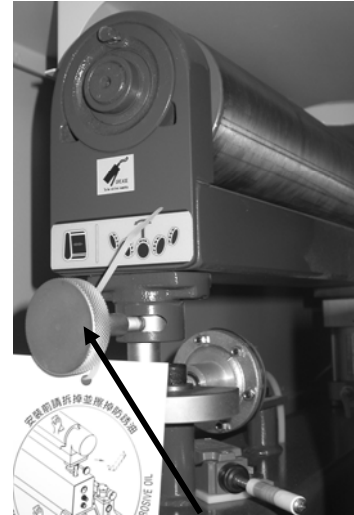
Sanding belt centralizing cam
