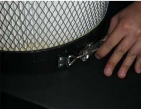
Figure 8: Releasing filter clamp
