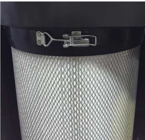
Figure 9: Hold canister from bottom when releasing clamp
