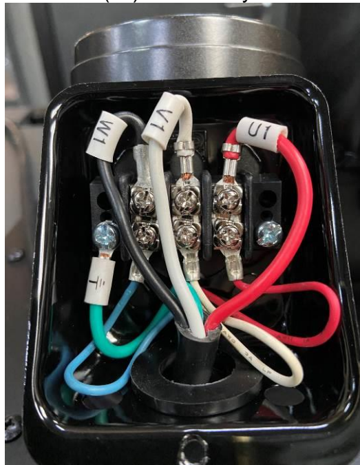
Figure 20: 220V Top Wiring in Junction Box
