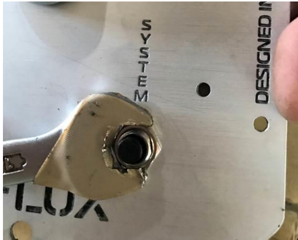
Figure 14: Replacing Overload Protector
