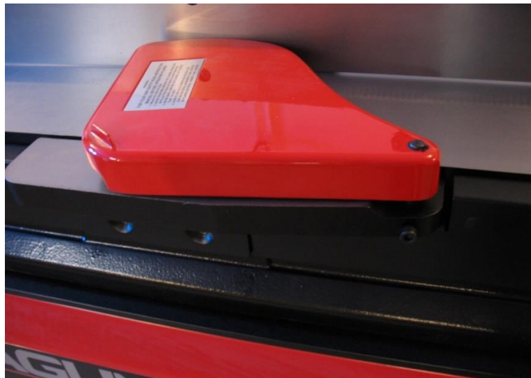
FIGURE 17: Cutterhead Guard installed
