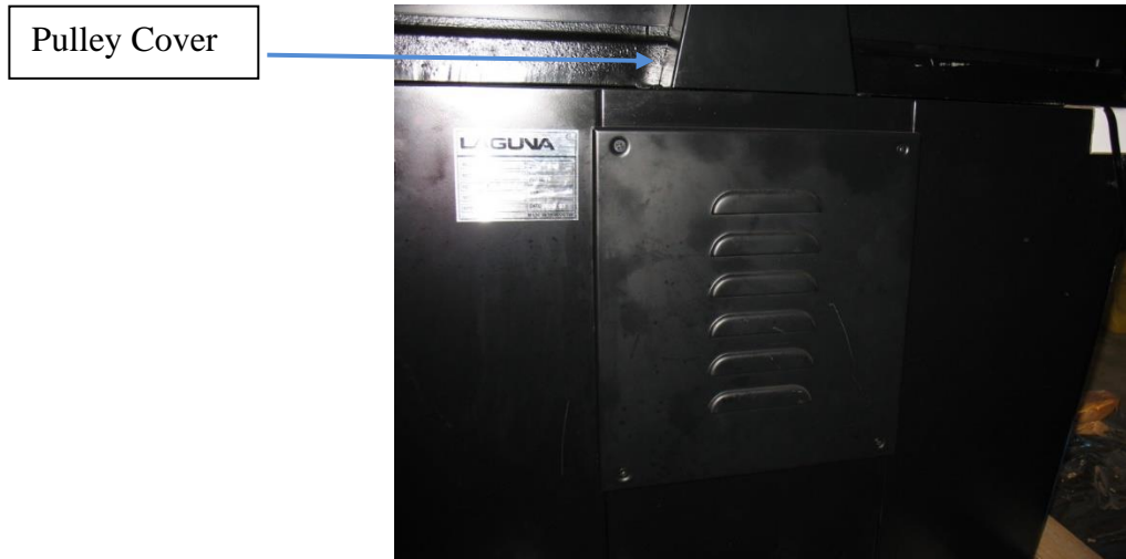
FIGURE 14: Pulley Cover installed
