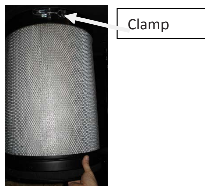
Figure 44: Hold canister from bottom when releasing clamp (top)
