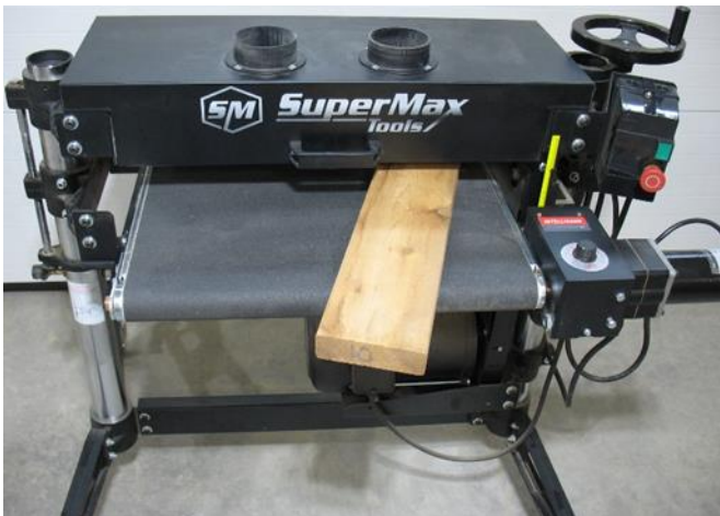
Fig. 15. Offset stock feeding angle.
