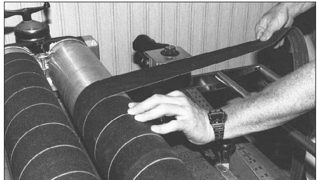
Fig. 10-e. Wrap around drum without overlap.
