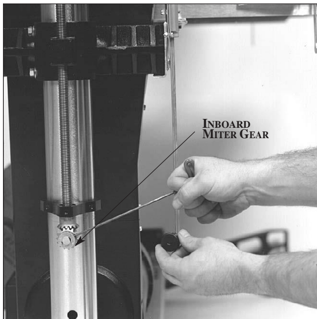
Fig. 6. Adjusting primary drum alignment.
