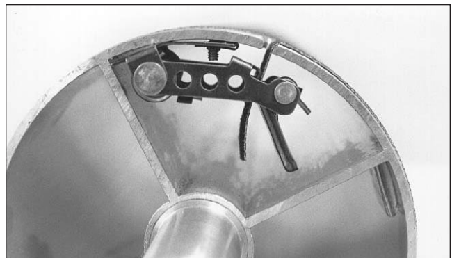
Fig. 10-i. Reset take-up as needed as wrap stretches.
