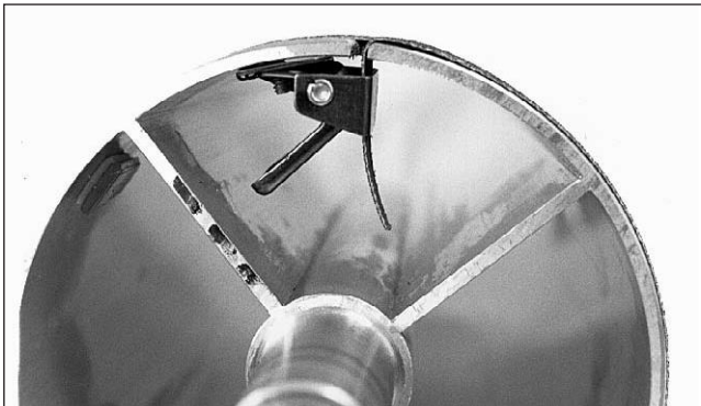
Fig. 10-d. Insert tapered end into outboard slot.
