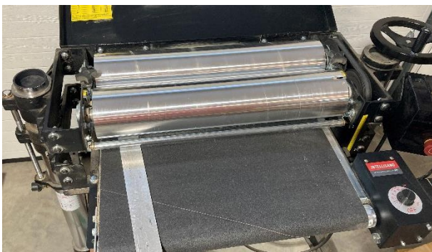
Fig. 4. Checking drum alignment (inboard side).
