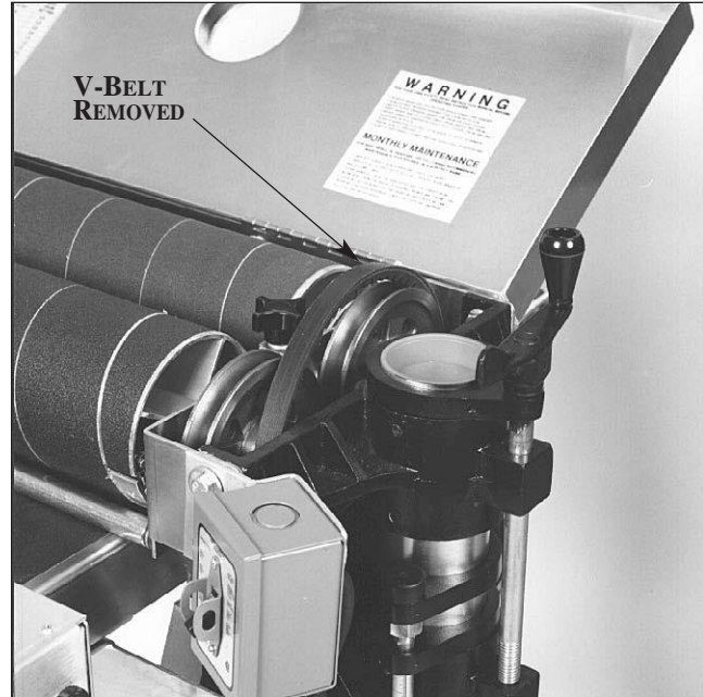
Fig. 30. Removing main motor V-belt drive.
