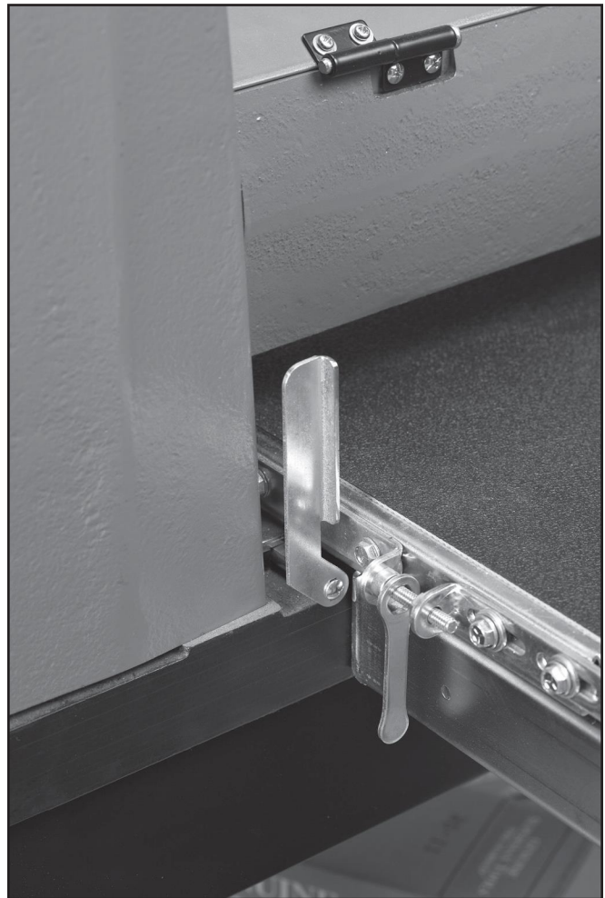
Fig. 9 Hanging wrench 1 of 2, for tracking conveyor
