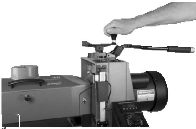
5 Raise the head of the sander by rotating the height adjustment handle up exactly one full turn.
