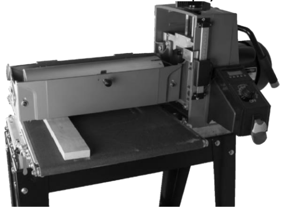
6 After the height has been adjusted move the piece of wood over to the outboard side (left) and lower the head by turning the handle down exactly one full turn until the DRO thickness matches what was noted in step #4.
