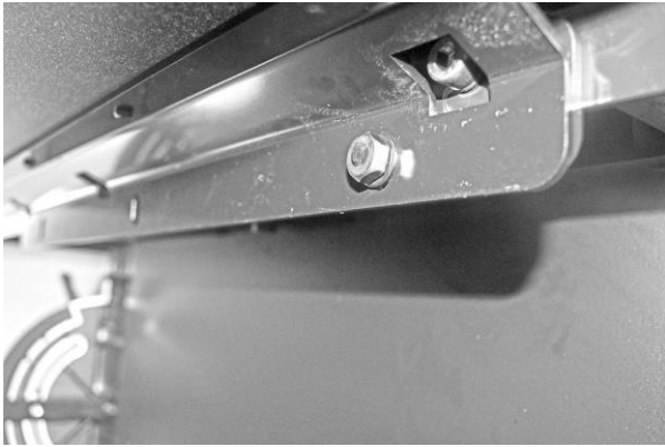
Bolt into thread holes:
