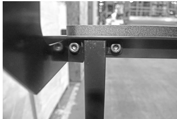
Hose support and Leg properly Installed:
