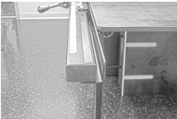
Front guide rail seated on front rail:
