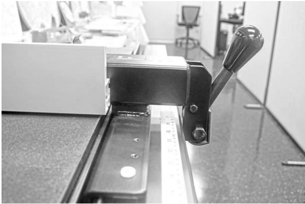
Fence fitted over the front guide rail
