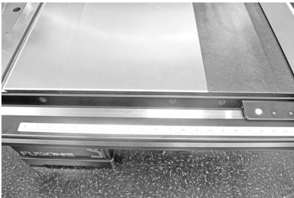
Front of rail showing counter sunk screws
