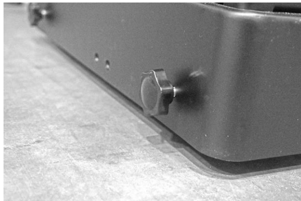
Loosening Lock Knobs
