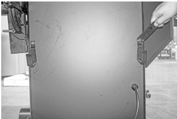
Fence Hook Installation
