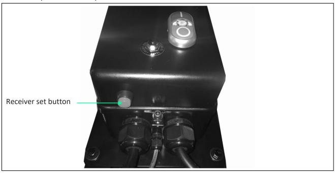
Figure 41: Programming remote control
