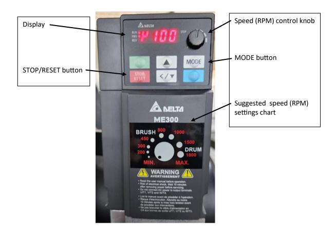
To turn "ON" the machine (drum or brush): Pull "ON" the safety paddle switch equipped on the conveyor control box to run drum or brush. The "RUN" button on the control panel of VFD is NOT programmed and does not control any functions.
