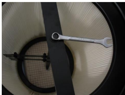
Figure 2M: Removing flap pivot bolt (from underneath)
