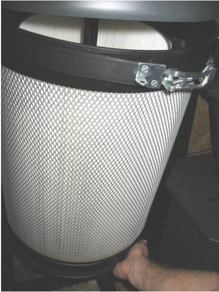
Figure 2N: Hold canister (from bottom) when releasing clamp (top)
