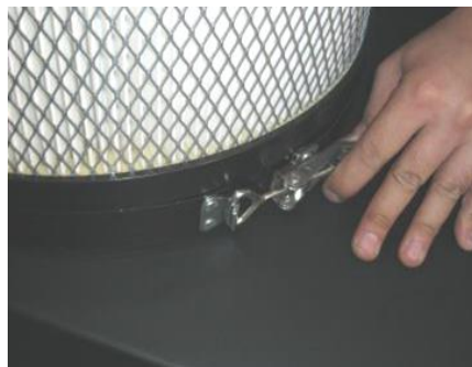
Figure 2M: Releasing collection bag clamp
