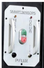
Fig. 2AA: Gen 1 Control Panel
