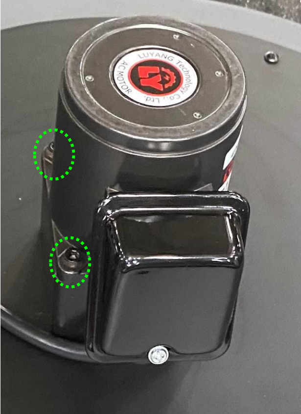
Figure 2U: Motor attachment bolts (2 of 4). Figure 2V: Auto clean motor
