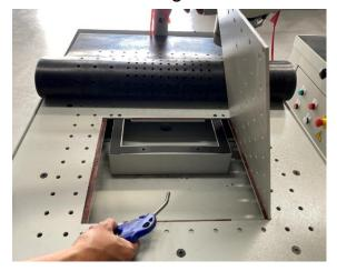
4. Replace the lids and fasten with screws, and place the rubber mat on the table after cleaning.
