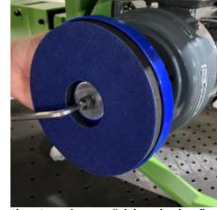
3. When installing a new brush, confirm the two large "drive holes" align with the two drive studs. See the image below, then hold brush tightly and use Allen wrench to tighten the bolt.
