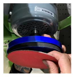
2. Change the abrasive holder: hold the abrasive holder tightly and use Allen wrench to turn clockwise to remove the bolt and the abrasive holder. Then, install new abrasive holder and use Allen wrench to turn the bolt
