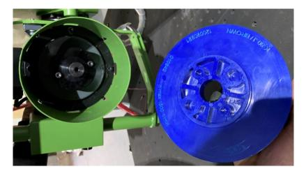
3. When installing a new brush, confirm the two large "drive holes" align with the two drive studs. See the image below, then hold brush tightly and use Allen wrench to turn the bolt clockwise to tighten the bolt.
