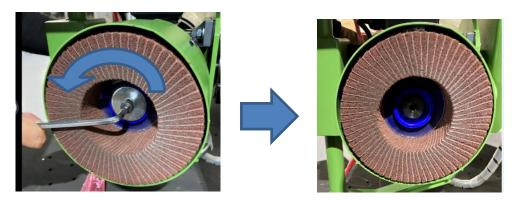
2. Remove the worn brush pieces from disc and replace with new brush pieces.
