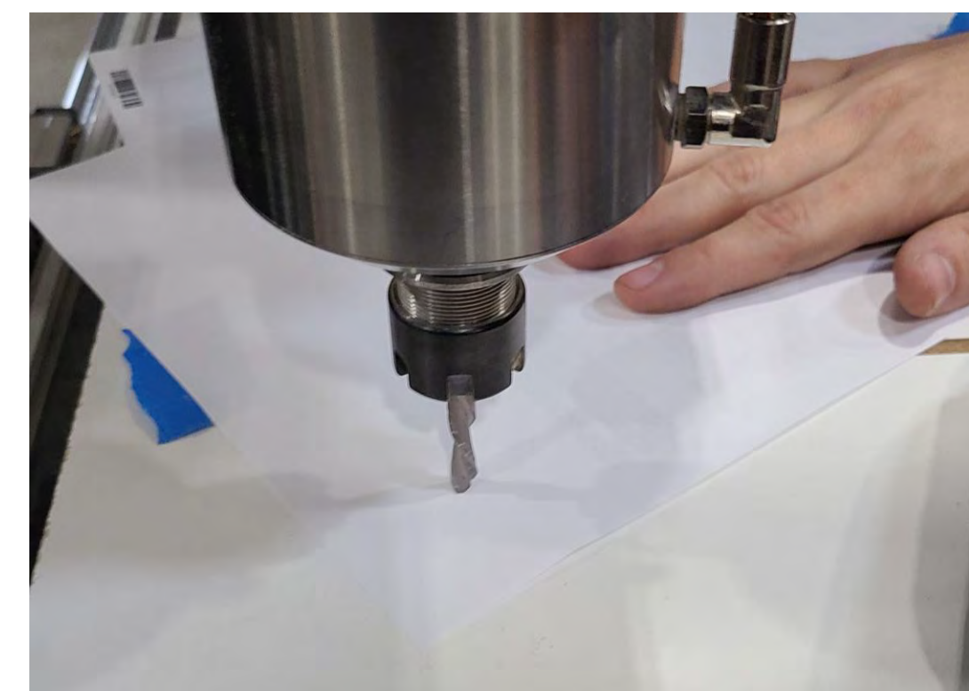
"Z-Zero Position with a piece of paper"
