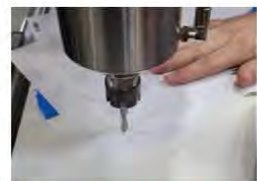
"Z-Zero Position with a piece of paper"
