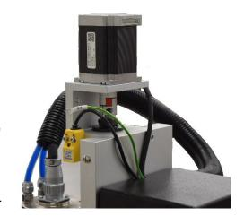
Figure 2-5: Stepper Motor
