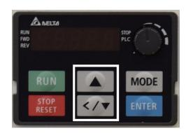
Figure 4-5: Adjust the RPM
