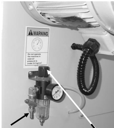
Air line connection
