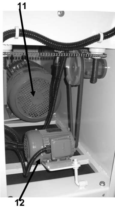
11. Main Motor/Sanding 12. Conveyor Lift Motor
