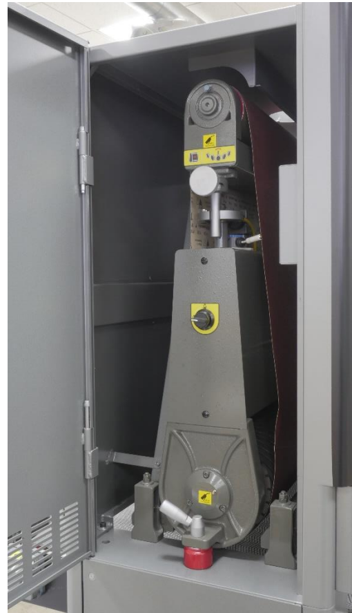
Abrasive sanding belt installed
