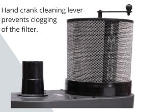
**The B|FLUX** comes standard with a 1 micron canister providing filtration of 99.97% of particles between 0.2 ~ 2 microns and features 17.2 square feet of polyester spun bond pleated filter to ensure maximum airflow.
