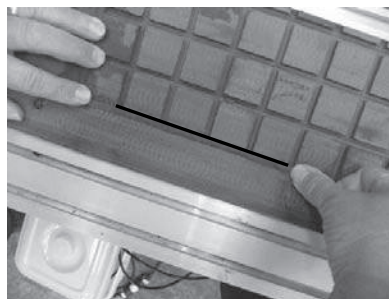
Inserting foam rubber gasket
