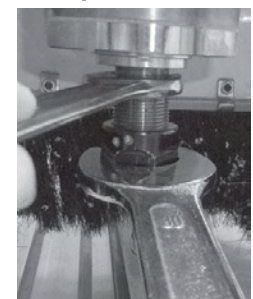
Tightening the spindle nut
