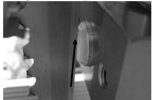
Rear blade guide shown with the side guides removed
