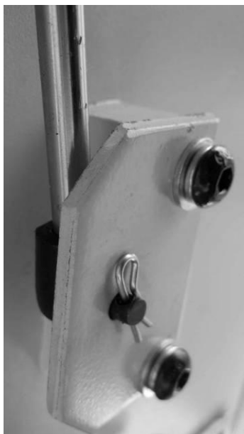
Gas assistor fitted to body
