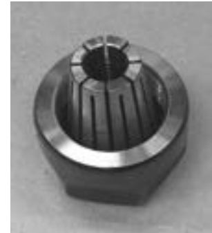
Collet fitted to spindle nut
