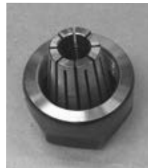
Collet fitted to spindle nut
