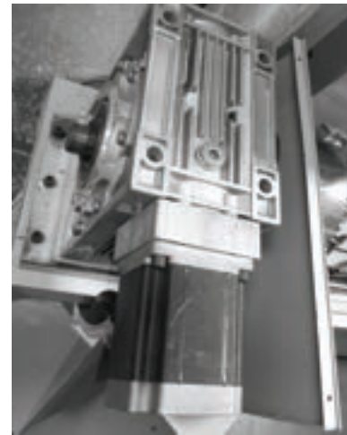
Chuck drive shown with the cover removed
