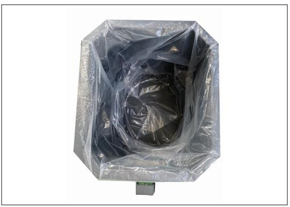
16. Place the drum insert inside the plastic bag (within the drum).
