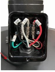
42. A qualified electrician must open the junction box on the auto clean motor and remove the strain relief at the bottom. Take the second motor cord leading from the top upright support with the control panel and insert into the strain relief, connect the wires according to the wiring diagrams on page 10 & 11. Close and secure the junction box after completing the wiring.
