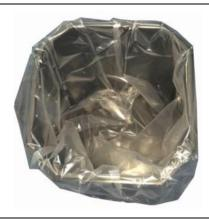
37. Insert the plastic debris collection bag inside the Octagon drum. Open and spread out the plastic bag to the corners and edges
