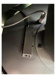
28. Attach the LED light to the drum lid using (6) M4x10mm Philip HD Bolt, (6) 3/16" flat washers and (6) M4 hex nuts.
