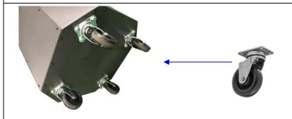
30. Assemble the Octagon drum. Locate the drum base panel, (it does not matter which side faces inside) and secure the (4) casters using (16) 5/16" x 3/4" hex bolts, (32) 5/16" x 1" flat washers and (16) 5/16" hex nuts.
