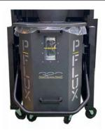
39. Lift the foot pedal bar. Align the Octagon drum window to the center point of the drum lid and push the drum in. Lower the foot pedal bar to seal the drum tight for normal machine operation.
