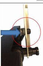
25. Secure the movable supporting brace on the foot pedal bar with the octagon foot pedal using (2) 3/8"x21mm hex bolts. Make sure the bolt head is on the inside of the octagon foot peddle. Adjust the tightness of this bolt accordingly. If this bolt is too tight, the Octagon foot pedal will not work smoothly. When too loose it will not pick up the Octagon drum.
