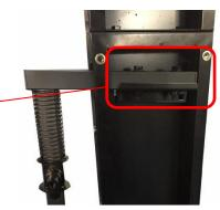
19. Secure the top end of the foot pedal bar to support bracket using (4) 5/16"x1-3/4" hex bolts, (8)5/16"x18x2mm flat washers and (4) 5/16" hex nuts. Make sure the foot pedal bar is pushed all the way to the end of the support bracket (indicated by yellow arrows). Follow the same steps for the opposite side.
