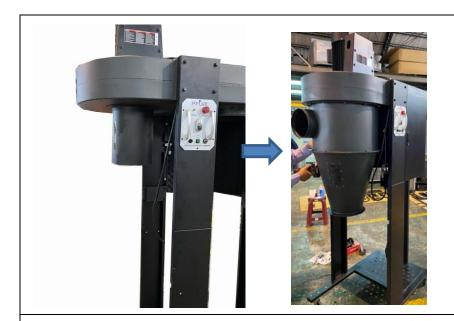
8. Attach the intake cylinder to the dust chute using (4) 5/16"x5/8" hex spring bolts. Then, attach the cyclone barrel onto the dust chute using (12) 5/16"x3/4" hex bolts and (12) 5/16"x18x2mm flat washers followed by attaching the cyclone funnel to the barrel using (12) 5/16"x3/4" hex bolts, (24) 5/16"x18x2mm flat washers and (12) 5/16" hex nuts.
