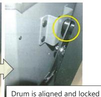
drum that both the left and rightside lift plates are over the topping on the foot pedal bar assembly before lifting the foot pedal bar up. When not aligned, the drum will not be fully sealed and will interfere with the air flow.
