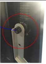
22. Attach the two ends of the Octagon foot pedal to the nut on the foot pedal bar.
