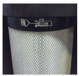
Figure 9: Hold canister from bottom when releasing clamp
