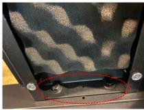
2. Remove the base which has been bolted to the (3) top upright supports. Keep the (6) 3/8"x3/4" hex bolts and (6) 3/8" flat washers for assembling the lower supports to the base. Keep the upper assembly lifted for step 5.
