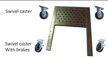
3. Turn base upside-down. Use (16) 5/16" x 3/4" hex bolts and (16) 5/16" flat washers. Attach the (2) 4" casters with brakes to the base. The casters with brakes should be attached to the side with the opening. The remaining (2) 4" swivel casters must attach to the other side of the base.
