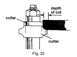
If the workpiece is to be shaped all around the perimeter, hold it firmly and push t he work straight into the cutter until t he dept h of cut is established by the collar as shown in Fig. 34. Continue to feed the work so that the point of contact on the edge is always 90 degrees to the collar (or directly in line with t he cutter edge) and held firmly against it.
