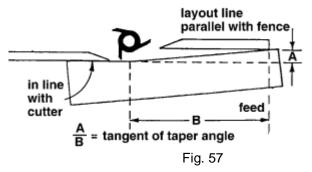
Caution: Do not use the standard fence for short work (12" or less in length on the side to be cut). Instead, use a miter gauge or special fixture to avoid losing control of the workpiece.
