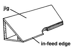
To perform a bevel-edge cut, the in-feed edge of the ig is placed against the infeed fence and clamped to the table as shown in Fig. 31. The outfeed fence is moved forward as necessary to compensate for the cut.
