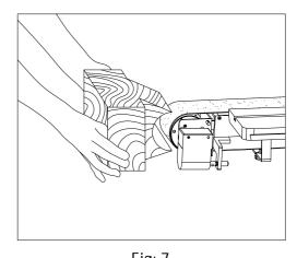
Fig: 7 FOR CONTOUR SANDING SEE FIG. 7
