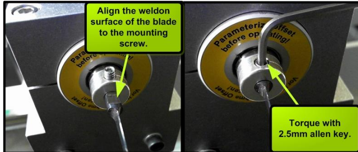
Figure 3. Changing blades on an EOT-2 module.
