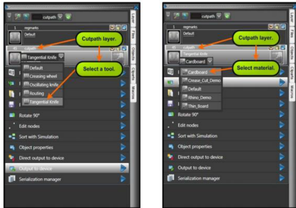
Figure: For each Cut path, a Tool and Material must be selected.
