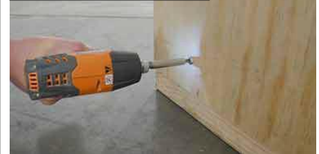
Unscrew the crate fasteners
