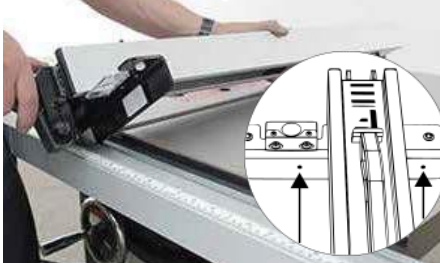
Position fence to access adj. screws
