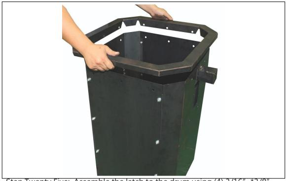
Step Twenty Five: Assemble the latch to the drum using (4) 3/16" \*3/8" round head thread bolts.
