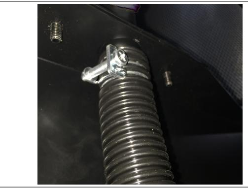
Step Twenty Nine: Place the vacuum suction ring inside before inserting the plastic bag in the Octagon drum.
