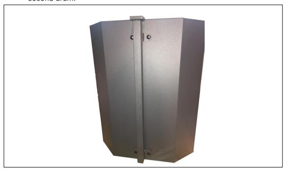
1.2. Take the one of the cover plates, (2) 1/4"\*1/2" carriage bolts, (2) 1/4"\*OD19\*2t flat washers and (2) 1/4" hex nuts and secure the cover plate to the opening on the top of the drum. For the bottom holes do the same, but first use foam tape to cover the square opening before bolting on the cover plate. Do the same to the second drum.
