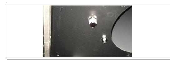
Step Nineteen: To adjust the distance of the sensor to detect the dust waste level use the white plastic pin that was provided in the hardware box.
