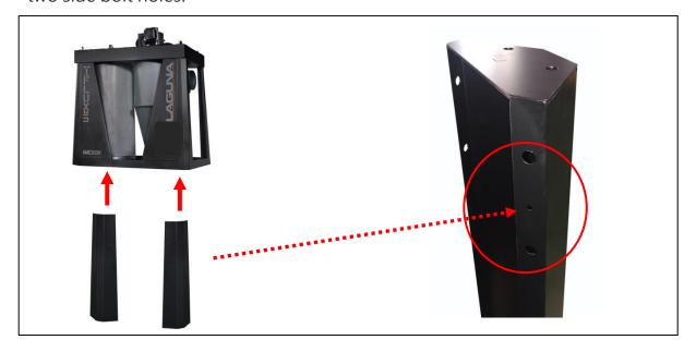
Step Three: Secure the (2) lower upright supports to the right side of the machine when facing the control panel. These two lower upright supports have a two dot marking on the side rim, as shown below. Use (4) 3/8" \*1" hex bolts and (8) 3/8" \*OD23\*2t flat washers and (8) 3/8" lock nuts for the two side bolt holes and use (1) M16\*50mm hex bolt for the center bolt.
