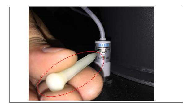
Step Twenty: Using the white plastic pin, insert the sharp point into the top end of the proximity sensor that is on top of the drum lid. You will find a small
