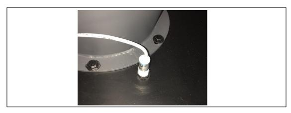
Step Eighteen: Make sure that the proximity sensor is not thread in too deeply into the drum lid. As this will create interference when the drum is inserted and may hit the proximity sensor creating damage.
