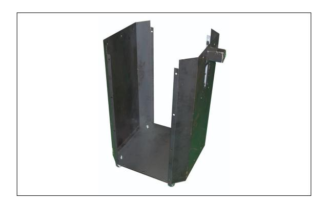
Step Twenty Three: Assemble the side panels to the drum using (6) 5/16" \*5/8" Philip hd bolts, (12) 5/16" \*OD18\*2t flat washers and (6) 5/16" nuts to secure the base. And then use (16) 5/16" \*5/8" Philip hd bolts, (16) 5/16" \*OD18\*2t flat washers and (16) 5/16" nuts to secure the panels to each other.
