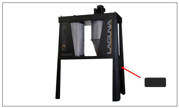
Step Seven: Secure the side horizontal panel to the left side of the unit; facing the control side. Use (12) 3/8" \*1" hex bolts, (24) 3/8" \*OD23\*2t flat washers and (12) 3/8" lock nuts.
