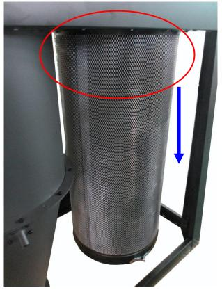
4. With the canister filter removed use a compressed air gun to thoroughly clean between the pleats, both inside and outside.
