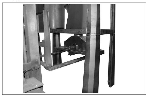
Step Fifteen: Secure the latch base plate to the front side of the drum lid using (2) 3/16" \*3/8" round head bolts.
