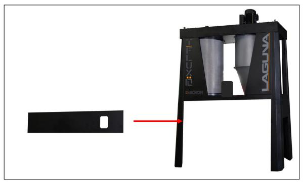
Step Five: Secure the back horizontal panel with the opening for the control panel to the front of the unit; facing the control side. Use (12) 3/8" \*1" hex bolts, (24) 3/8" \*OD23\*2t flat washers and (12) 3/8" lock nuts.
