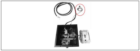
Step Seventeen: First remove one of the black screws off the sensor then thread the sensor through the hole on the drum lid. Take the black screw and tighten the other end of the sensor that is on the inner side of the lid.
