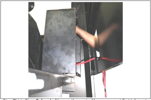
Step Thirty Five: Before bolting on the control box, you must first take out the control panel from the box and insert through the hole on the horizontal panel.
