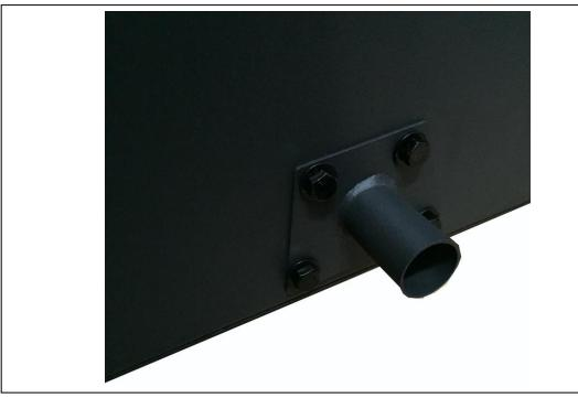
Step Twenty Seven: Attach the  $\emptyset1$ -1/4" x0.8M black flex hose to the drum vacuum suction tube and use the  $\emptyset1$ -1/4" hose clamp to tighten and secure the black flex hose in place.
