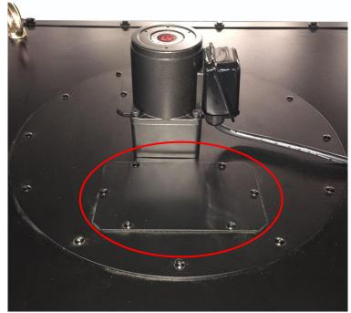
2. Loosen the bolt off of the rotation shaft as shown below. Set the shaft aside for later use. Keep the bolt for use when reassembling the rotation shaft.
