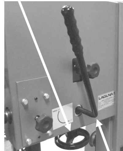
Quick action blade tension lever (activated)
